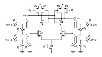
Figure 4. Charge Sharing Comparator for stage ADC
