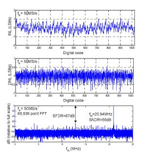
Figure 9. INL, DNL, FFT of output, f<sub>s</sub>=50MS/s
