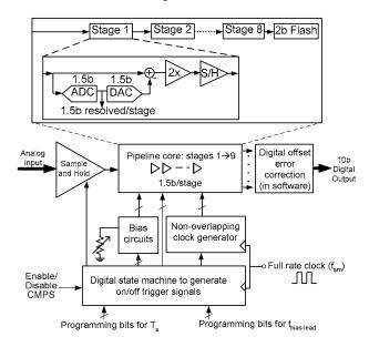
Figure 2. System Level diagram of Pipelined ADC
