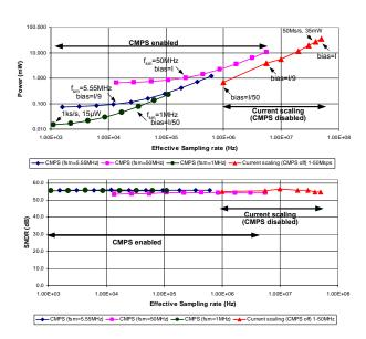
Figure 8. Power & SNDR vs.  $f_s$  for  $f_{sm}=1$ , 5.55, 50MHz
