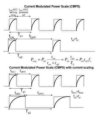
Figure 1. Current Modulated Power Scale (CMPS)
