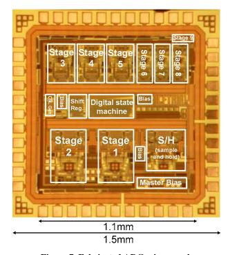
Figure 7. Fabricated ADC micrograph
