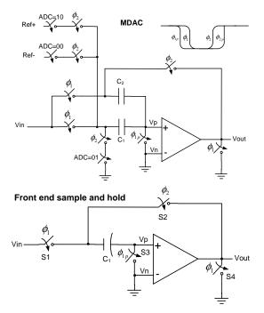
Figure 5. Stage MDAC, Front end Sample and hold
