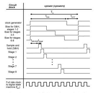
Figure 3. Power on/off timing of blocks in ADC
