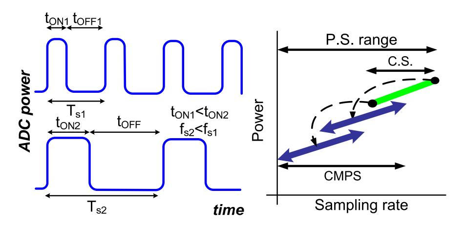
Variable t<sub>ON</sub> (f'n of I<sub>B</sub>), variable t<sub>OFF</sub> to realize different f<sub>s</sub>
