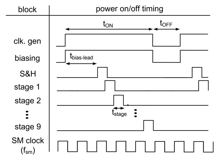
bias circuits powered on first due to slow power on times
