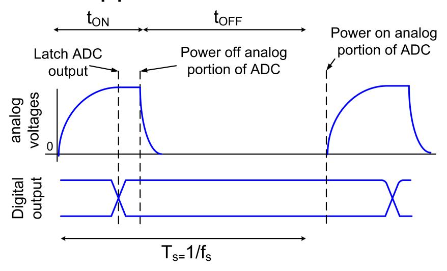
Analog power only during t<sub>ON</sub>, digital power during digital output transitions (dynamic power)
