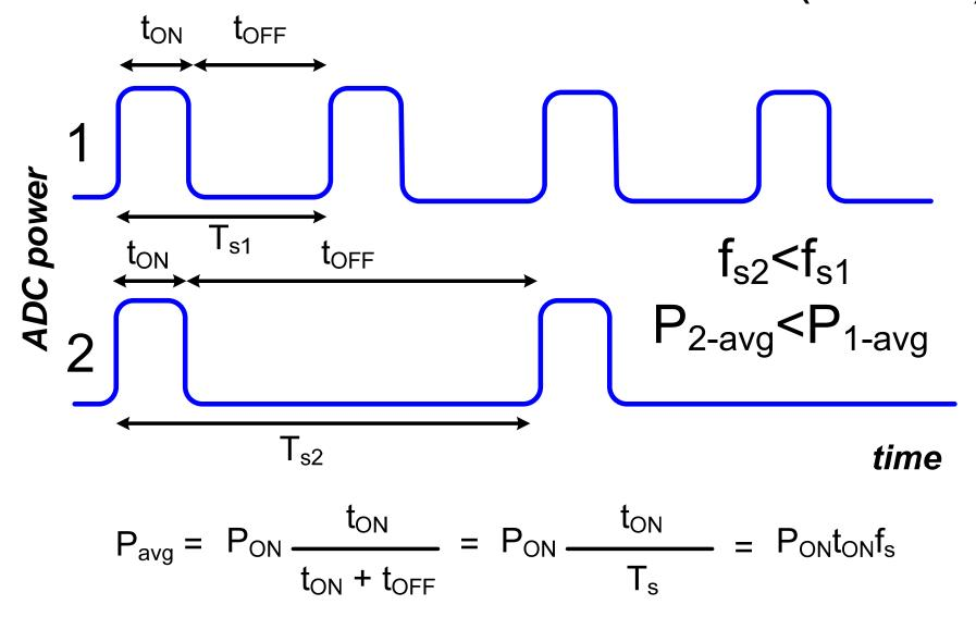
Constant t<sub>ON</sub>, variable t<sub>OFF</sub> to realize different f<sub>s</sub>
